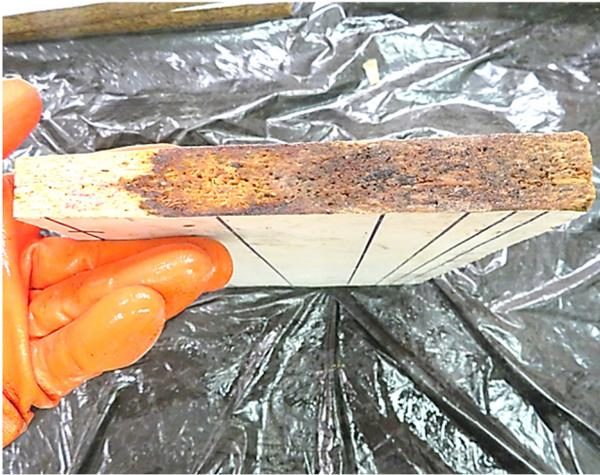
**Photo 11** Vinyl-faced particleboard moisture adsorption in ambient RH, 6 cycles.
