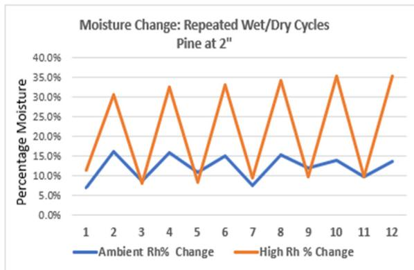
Fig. 2 Moisture content at 2" above the source in pine specimens exposed to cyclical wet/dry conditions.
