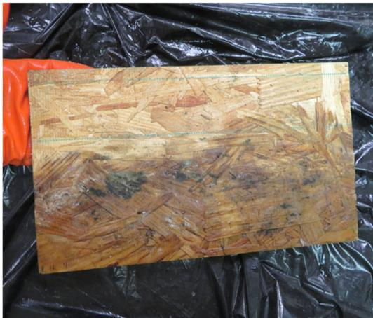
**Photo 9** OSB moisture adsorption in ambient RH, 6 cycles.
