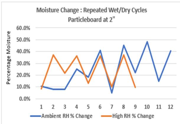
Fig. 8 Moisture content at 2" above the source in particleboard specimens exposed to cyclical wet/dry conditions.
