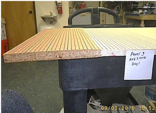
Photo 1 Thickness swell in 5/8" particle board.
