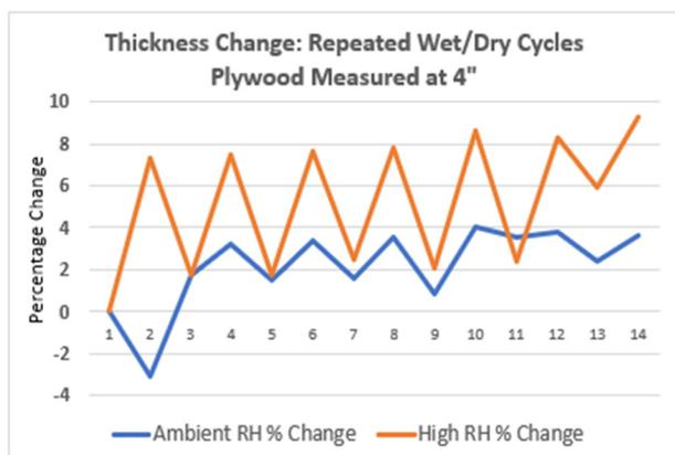
Fig. 13 Thickness measurement changes in plywood specimens exposed to cyclical wet/dry conditions at 4".
