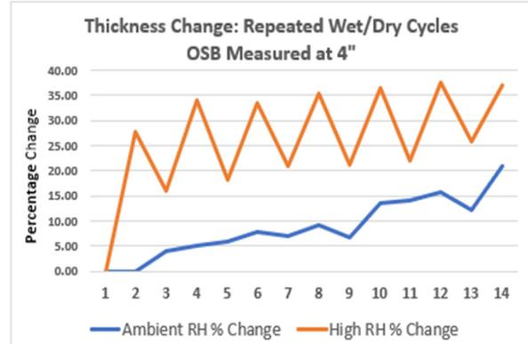
Fig. 15 Thickness measurement changes in OSB specimens exposed to cyclical wet/dry conditions at 4".
