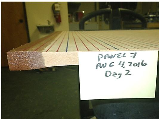
Photo 2 Thickness swell in 3/8" medium density fiberboard.
