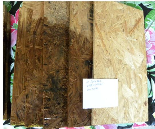
**Photo 10** OSB moisture adsorption in high humidity, 6 cycles [5].
