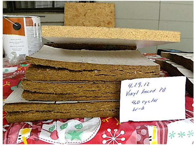
**Photo 12** Vinyl-faced particleboard moisture adsorption in high humidity, 4 cycles [5].
