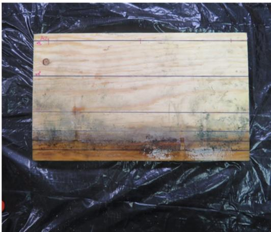
Photo 5 Solid pine moisture adsorption in ambient RH, 6 cycles.
