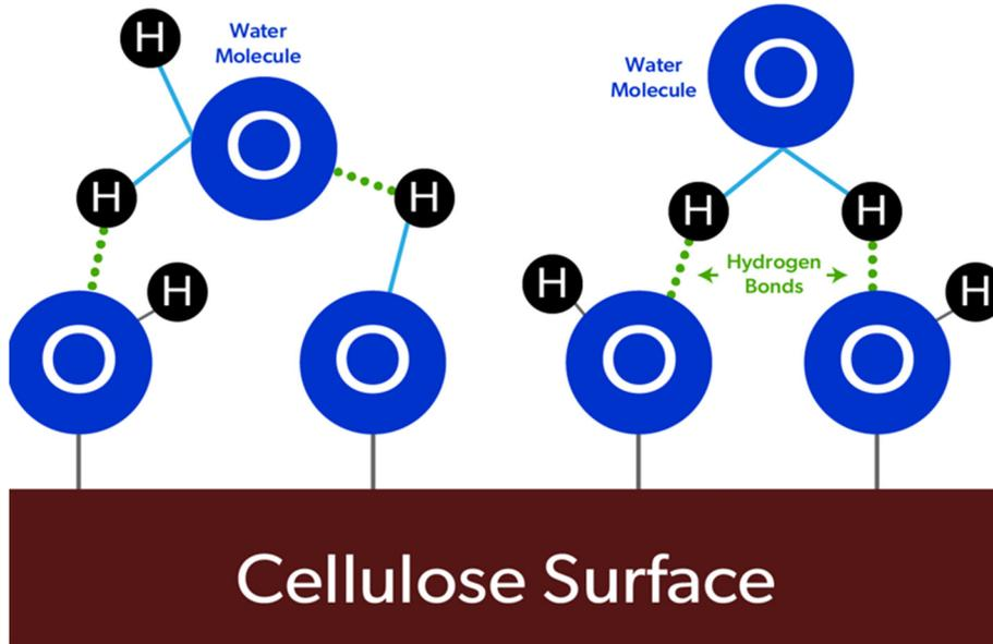
Fig. 1 Cellulose molecule with exposed hydroxyl molecules. Exposure to water molecules allows hydrogen bonds to form between the hydroxyl and water molecules.
