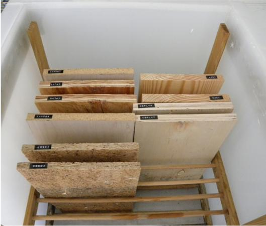
**Photo 3** Closed test apparatus with the polyethylene lid removed.
