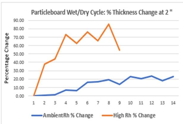
Fig. 16 Thickness measurement changes in particleboard specimens exposed to cyclical wet/dry conditions at 2".
