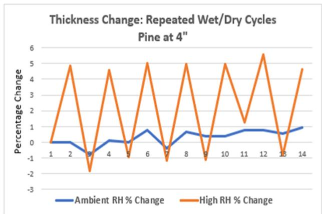
Fig. 11 Thickness measurement changes in pine specimens exposed to cyclical wet/dry conditions at 4".
