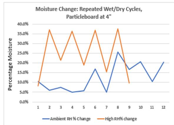
Fig. 9 Moisture content at 4" above the source in particleboard specimens exposed to cyclical wet/dry conditions.
