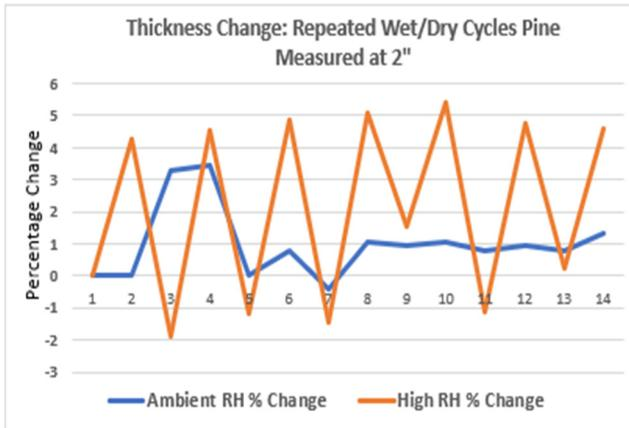
Fig. 10 Thickness measurement changes in pine specimens exposed to cyclical wet/dry conditions at 2".
