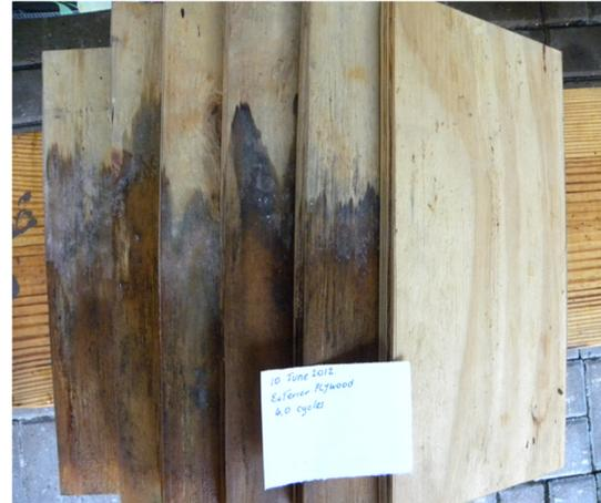
**Photo 8** Plywood moisture adsorption in high humidity, 6 cycles [5].
