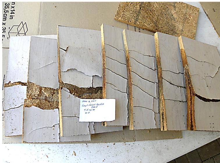
**Photo 13** Vinyl-faced particleboard moisture adsorption in high humidity, 4.5 cycles [5].
