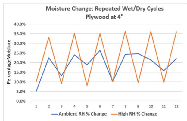
Fig. 5 Moisture content at 4" above the source in plywood specimens exposed to cyclical wet/dry conditions.
