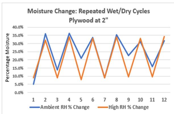
Fig. 4 Moisture content at 2" above the source in plywood specimens exposed to cyclical wet/dry conditions.
