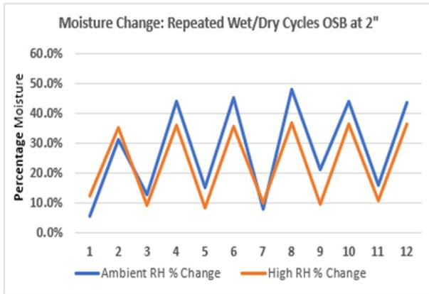
Fig. 6 Moisture content at 2" above the source in OSB specimens exposed to cyclical wet/dry conditions.
