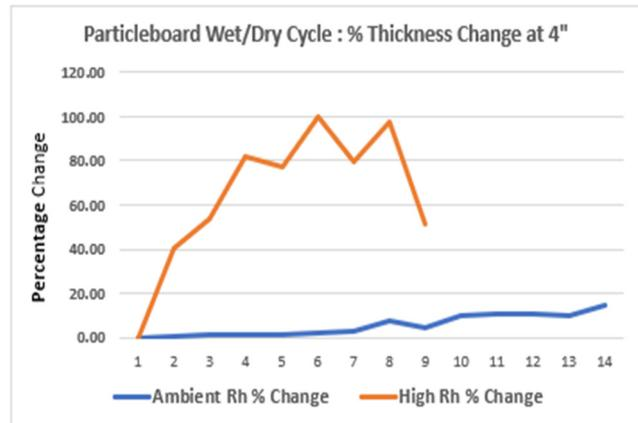
Fig. 17 Thickness measurement changes in particleboard specimens exposed to cyclical wet/dry conditions at 4".
