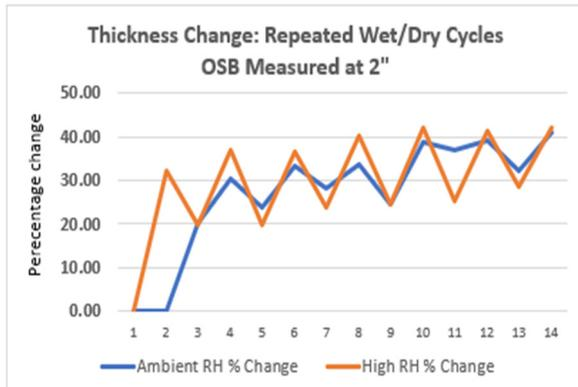
Fig. 14 Thickness measurement changes in OSB specimens exposed to cyclical wet/dry conditions at 2".
