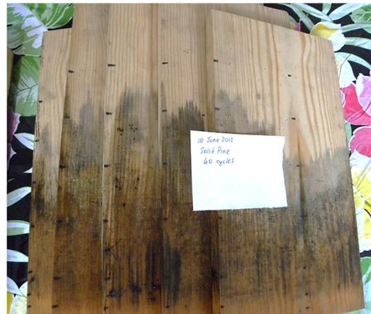
Photo 6 Solid pine moisture adsorption in high humidity, 6 cycles [5].
