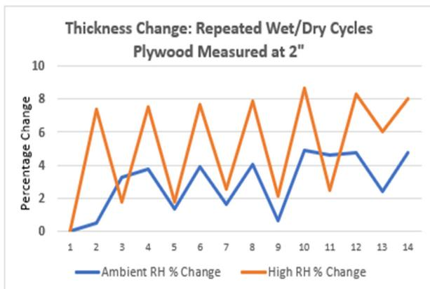
Fig. 12 Thickness measurement changes in plywood specimens exposed to cyclical wet/dry conditions at 2".
