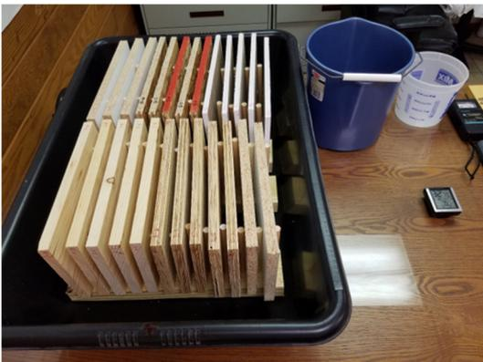
**Photo 4** Open test apparatus exposed to ambient temperature and RH conditions.
