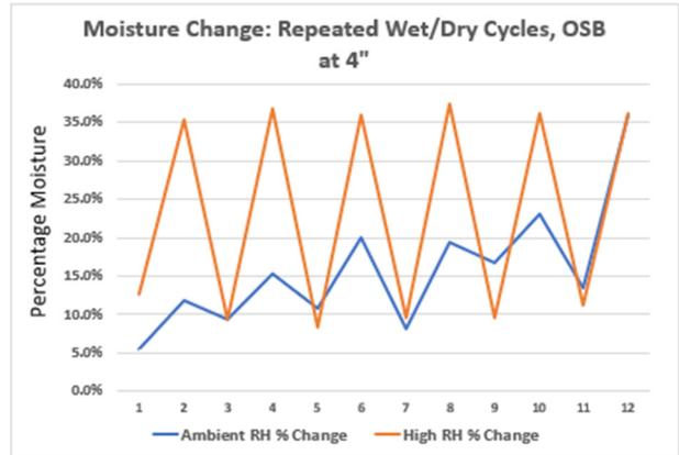
Fig. 7 Moisture content at 4" above the source in OSB specimens exposed to cyclical wet/dry conditions.
