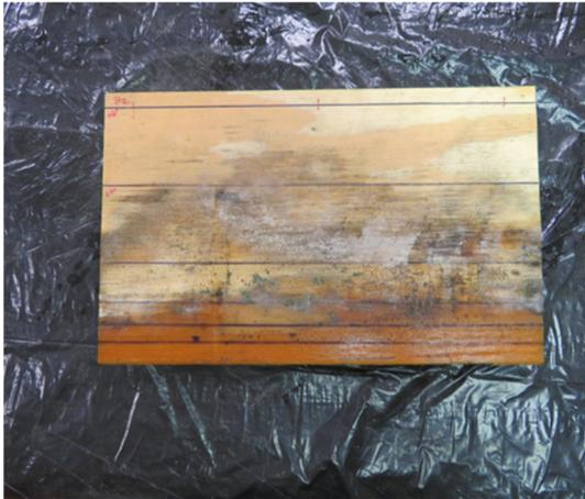
**Photo 7** Plywood moisture adsorption in ambient RH, 6 cycles.
