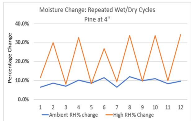
Fig. 3 Moisture content at 4" above the source in pine specimens exposed to cyclical wet/dry conditions.
